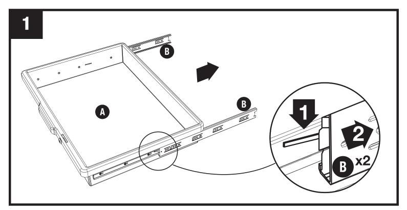
Pull drawer slides (B) out of drawer (A) as far as they can be pulled out. Push lever up or down to release drawer slide (B) from the drawer (A) completely. Repeat on the other side. Set drawer aside.
