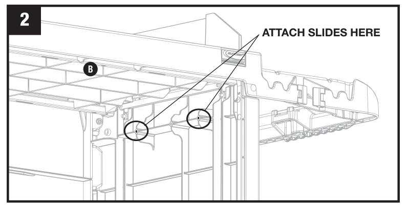
Screws will go through holes in slides and insert into these two hole locations on side panels.
