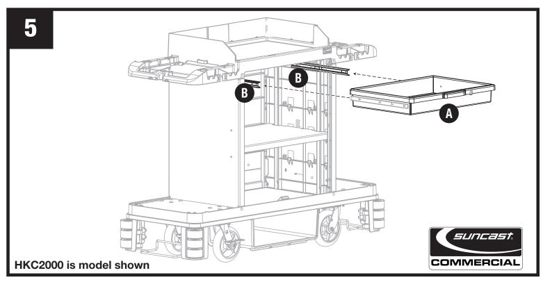
Pull slides (B) out of cabinet. Slide the drawer (A) into ends of drawer slides (B) located inside cart and slide all the way in to lock.
