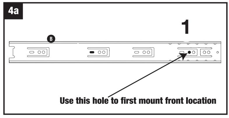
IMPORTANT: Inner slide has been removed for clarity.
