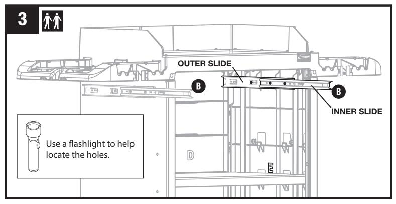
Attach slides (B) into inside of panels as shown using three screws (E). **IMPORTANT:** Slide away inner slide to expose appropriate screw holes. See step 4 for correct screw locations.
